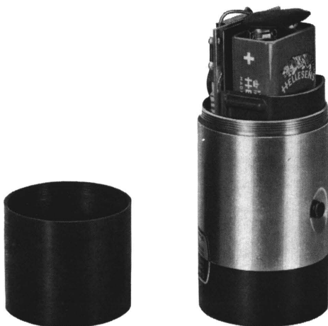
Fig. 2.4. Insertion of 9 V-battery in the Calibrator.
